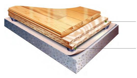
Two Layers 15/32" (12 mm) Plywood Subfloor or "HPS" (Hardwood -Premium Sheathing)
