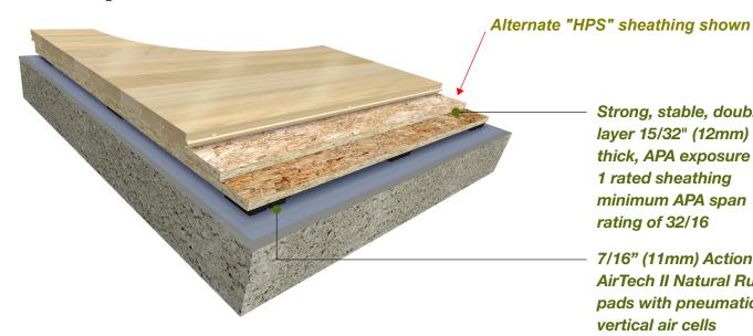
Strong, stable, double layer 15/32" (12mm) thick, APA exposure 1 rated sheathing minimum APA span rating of 32/16
