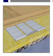
KTL SPORT PORTABLE PRO SUMMIT V2 SYSTEM is an area-elastic sports floor, based on 7/8" (22mm) solid hardwood 8-strip or multi-strip panels, laid floating in a brick pattern on an existing sports floor or on levelled concrete. The panels connect to each other on all sides by means of the unique flexi-lock system. The panels come with a supporting full plywood underlay. Total construction height including KTL 3/8" (10mm) sports foam strips is 1-3/4" (44mm) including full 1/2" (12mm) plywood layer.
