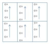
Roll material is stretched slightly during the manufacturing process. At the job site, the installer should unroll all cuts and allow to relax overnight. A bare minimum of two hours is required. Shaking the material once it is unrolled can help it to relax.
